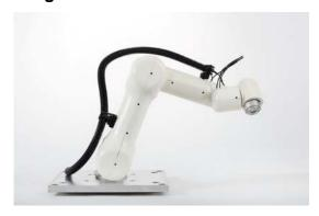
Collision protection from Mayser: pressure-sensitive and capacitive arm and joint safety solutions protect humans from or during contact with robots.
