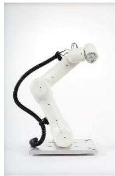
3D collision protection from Mayser: pressure-sensitive and capacitive arm and joint safety solutions protect humans from or during contact with robots.
