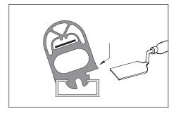
Repeat these 3 steps for the next 40 - 80 cm until the entire rubber profile is fitted to the C-rail.
