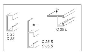
Apart from rails C 35 M and C25 M, the rails illustrated on the left are also available. Simply drill holes at the arrows and attach them to the closing edge
