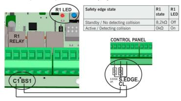
The equipment can be connected to the control panel with input for 8k2 / 10k safety edge or directly into a safety input normally closed contact as if it were a photocell or stop signal.
