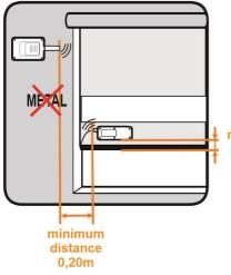
Do not place metal surfaces between transmitter and receiver. For maximum range, both the receiver and transmitters must be installed with the same orientation (vertical or horizontal).
