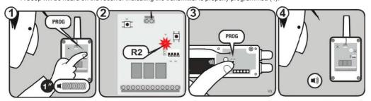
•To exit programming mode, wait for 20 seconds or press PROG button on the receiver. Two beeps will be heard.
