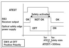
When working with optical safety edges, in ON mode, only OSE-S7502B and OSE-S7502 are allowed as they are kept always active. The radio communication is tested every 7 or 30 seconds depending on the selector SW1 of the receiver. In WORK mode, the ATEST signal is used to power up and down the optical safety edges. The radio communication is tested as in ON mode and when the optical elements are powered up and down.
