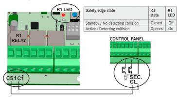
Example: connection to control panel with input for 8k2 / 10k safety edge
