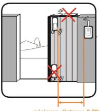
In installation likely to have communication cuts between the transmitter and the receiver, the antenna must stand vertically from the hole in the gland.
