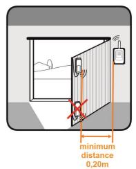
Do not fit the device at ground level
