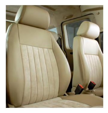
INDUSKIN as a 2D stamped part of open cell PU-ether foam functions as a base material for seat heating systems in climatised seats. In the embossing process, the base material is provided with the required seat contour (seat piping). Use of filter foam enables optimum ventilation and aeration of the heated leather seats.
