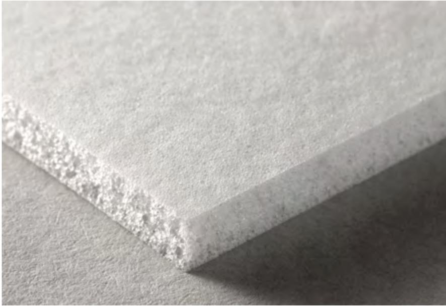
MAYSER BLUEFOAM® DG-T is an aliphatic polyester polyether polyurethane coating foam with excellent properties for versatile use in products with long-lasting skin contact (derma grade, DG).
