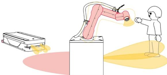
Various safety components such as safe ultrasonic sensors, surface sensors, pressure-sensitive and capacitive collision protection as well as soft cover for safe cobot working environments (HRC)
