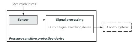
If you combine sensors with control units and thereby place pressure-sensitive protective devices on the market, you should observe the basic requirements according to ISO 13856.
