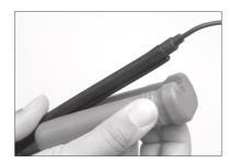
6. Proceed in the same manner at the other end of the contact profile using a resistor end piece (EKS/W) or another cable end piece (EKS/BK).
