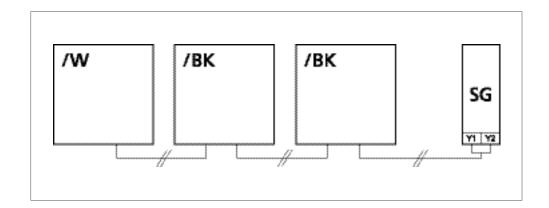
Sensor /BK: 4-wire-technology wired straight to the control unit
