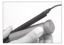
6. Proceed in the same manner on the other end of the contact profile with a resistor end piece (EKS/W) or another cable end piece (EKS/BK).
