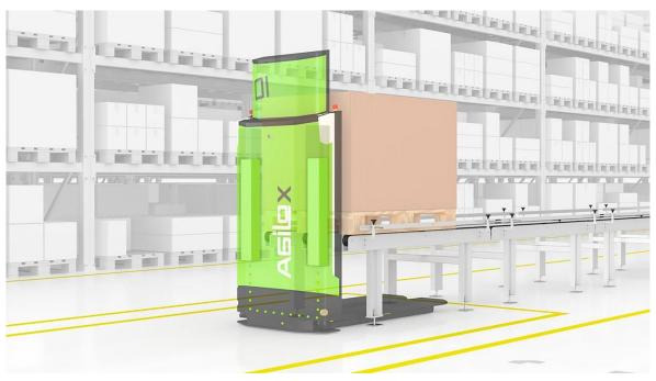
Agilox conveyor systems rely on ultrasonic sensors for trouble-free manoeuvring in tight spaces
