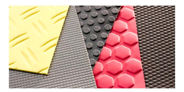
By hot embossing, surfaces of polyurethane soft foam materials are embossed. Tools are produced according to customer requirements.
