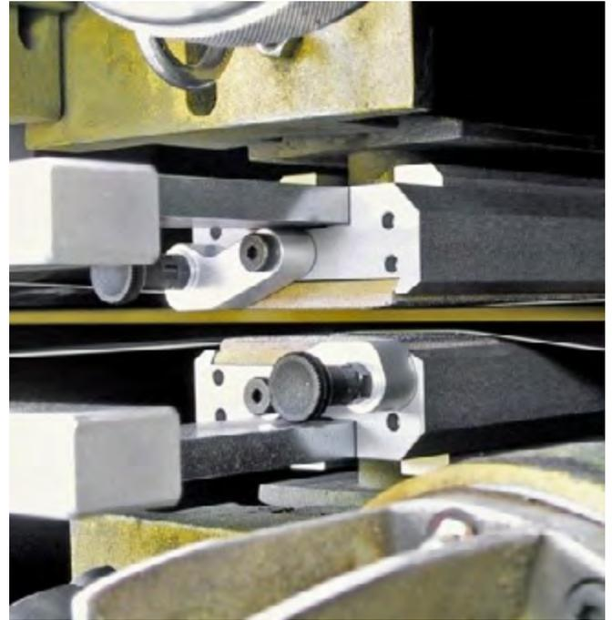
INDUCON® has very good resilience and hardness which is adjustable in narrow tolerances. It is therefore used as an accessory for grinding machines in the sheet producing industry. The compensating, durable material is used as support padding in the grinding shoes of grinding machines and makes an important contribution to a perfect surface finish in the production of wooden and plastic sheets for the furniture industry. In addition, it is used as an elastic base in pad printing.
