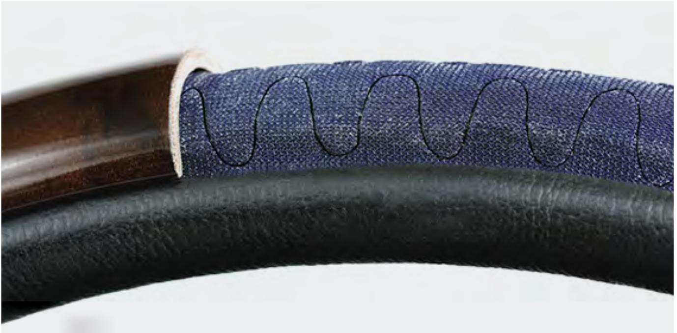
INDUCON® is a compensating material with adjustable haptics and is used as a base material for steering wheel heating systems. The main focus is on ensuring that the heating wire in the leather-covered steering wheel cannot be seen or felt. In addition, the smooth INDUCON® surface ensures economic use of adhesive when coating.
