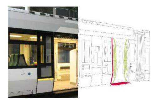
To ensure maximum passenger safety and trouble-free operation, Mayser has developed a capacitive sensor: the Non-Touch Detection System.
