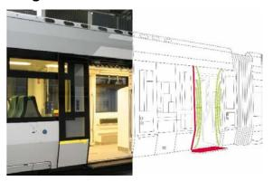
The Non-Touch Detection System only reacts to movements in the immediate critical area of the sensor, along the main closing edge.
