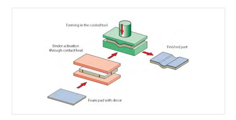
Pressed three-dimensional moulded parts offer excellent dimensional stability with a low weight. In addition, special substrate materials offer very good acoustic properties. Depending on the required edge design, a waterjet trim or the bending process is used. The wide variety of materials, decorations and processes enable an attractive design and a high level of product individuality.
