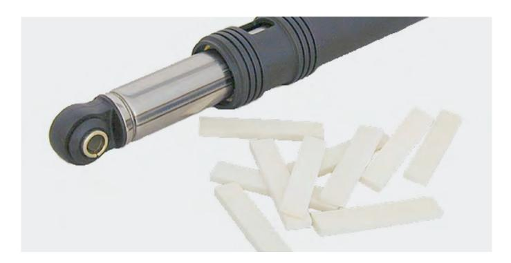
INDUCON® is used as a friction coating for friction dampers. Due to the exactly controllable hardness of the material, the frictional force of the damper can be adjusted in a wide range. The narrow thickness and weight tolerances of the material enable a narrow tolerance range of the finished product and optimum use of material.
