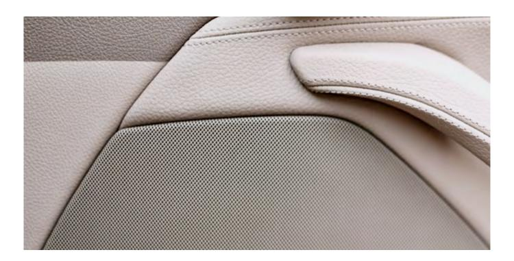
Surface-compressed polyurethane-polyether foam materials are used as coating foams for leather interior parts. Our production process smoothes the foam surface. The adhesive coating prevents formation of typical orange peel effect and gives the finished component a high quality surface quality.
